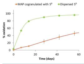
Figure 4. Effect of co-granulation of elemental S (S<sup>0</sup>) on the rate of oxidation in soil (pH(water) 5.6, 3.8 %OM) at 25°C (77°F) and where particles (17  $\mu$ m diameter) were dispersed throughout the soil or co-granulated with monoarmonium phosphate (Mosaic Fertilizer Technology Research Centre, unpublished data).
