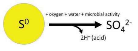
Figure 1. The reaction of elemental S (S<sup>0</sup>) oxidation in soils to sulfate (SO<sub>4</sub><sup>2-</sup>).
