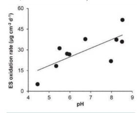
Figure 2. Effect of soil pH on oxidation of elemental S (ES) across ten soils at 25°C (77°F) where particles (average diameter 48  $\mu$ m) were dispersed through soil. The line represents: Rate = 6.29 pH<sub>water</sub> - 12.7 : r = 0.75, P <0.05 (Zhao et al. 2015).
