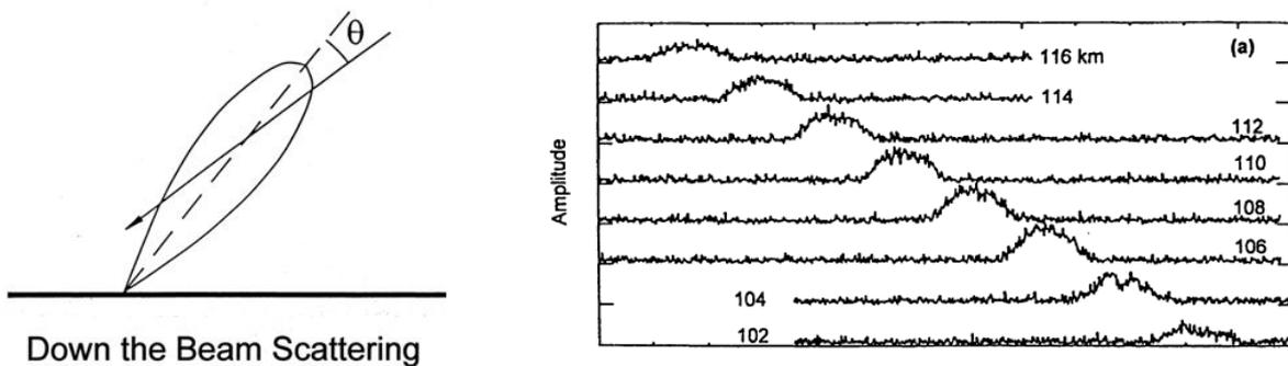
Figure 16. The ionisation from a particle moving down the beam detected in successive range bins.
