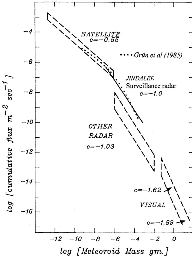
Figure 15. Flux of particles incident on the Earth for a large range of masses. Only radar observations at 6 MHz frequencies or less are consistent with satellite and optical observations
