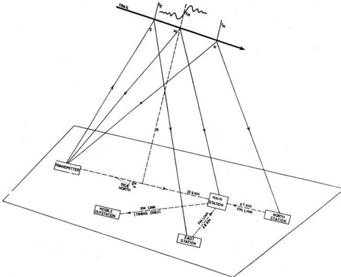
Figure 7. The multi station system used to determine meteor orbits and study atmospheric turbulence in 1961.
