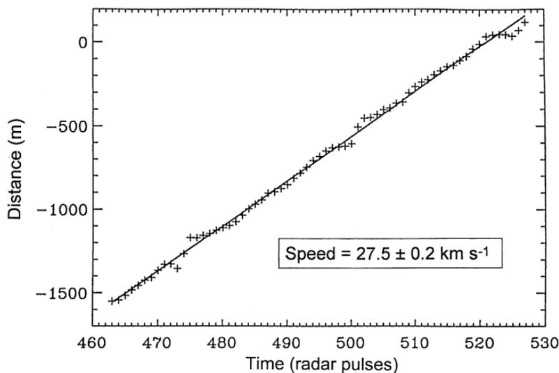
Figure 12. Distance back along the trail from the  $t_0$  point (see figure 2)
