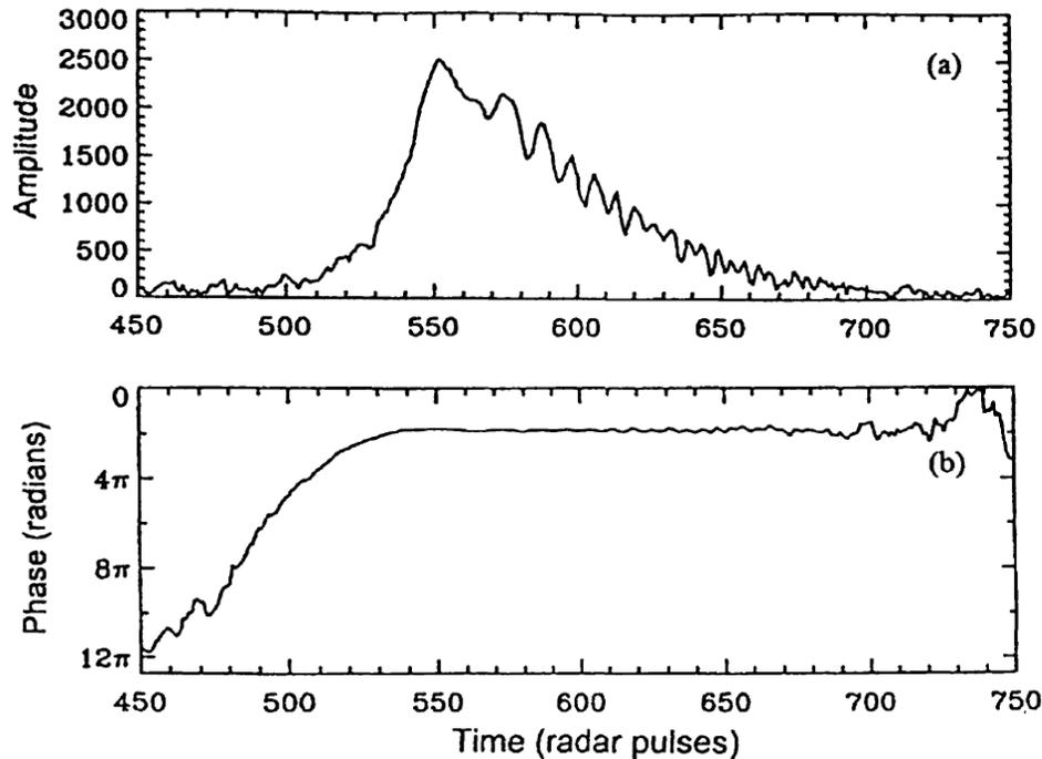
Figure 11. Amplitude and phase of a meteor echo observed with the narrow beam 54 MHz radar.
