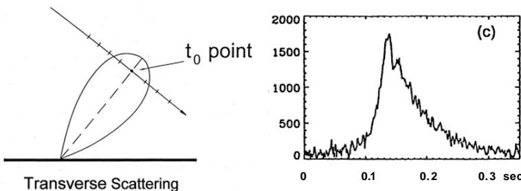
Figure 2. Typical radar echo from a meteor trail
